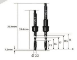
Tapered drills have V-shaped tips, for better correlation with the implant, 3 cutting edges offer good stability. The tapered shape reduces frictional heating. Variable helix for enhanced drilling control and twisted flute for bone extraction.
